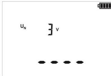
The meter is ready for measurement. Value of interference voltage is displayed on the auxiliary display.
