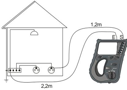
Connect the measured object to terminals **S** and **E** of the meter.
