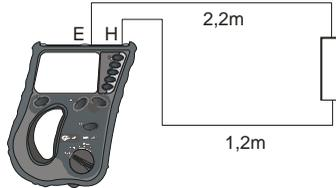
Connect the measured object to terminals **E** and **H** of the meter.
