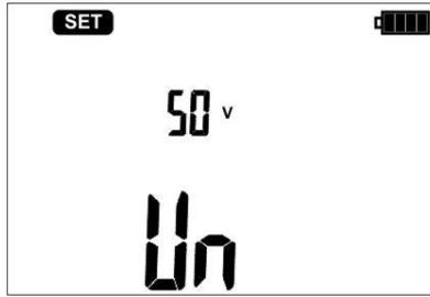
Using  $U_N$  button set test voltage on 25V or 50V. After 5 sec. the meter returns to the measurement mode. You can also confirm the choice by pressing the **START** push-button.
