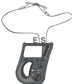
Short the test leads by putting crocodile clips on exposed ends of the test leads.
