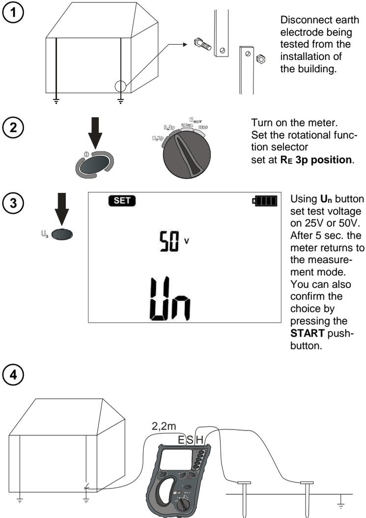
The current electrode (driven into earth) should be connected to **H** socket of the meter. The voltage electrode (driven into earth) should be connected to **S** socket of the meter. The earth electrode being tested should be connected to **E** socket of the meter. The earth electrode being tested and the current electrode and the voltage electrode should be located one line
